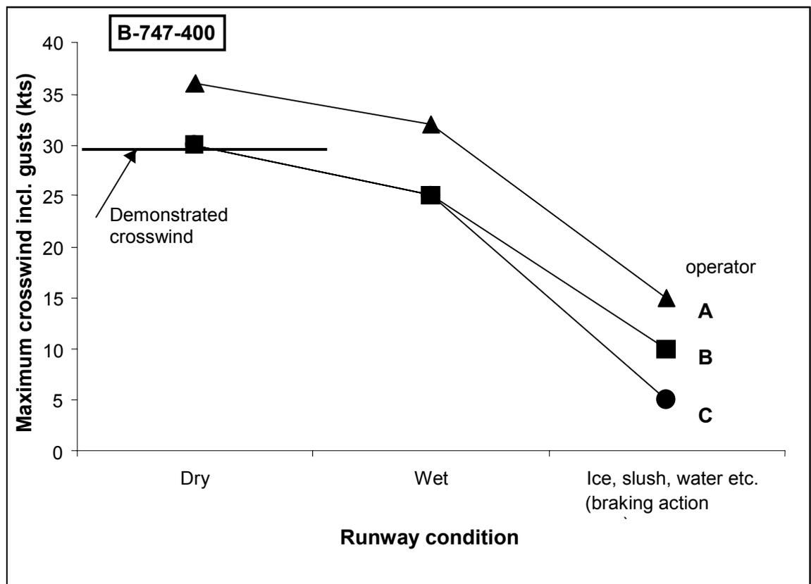
Figure 6: Maximum crosswind of a B-747-400 for landing as function of runway condition for three different operators.
